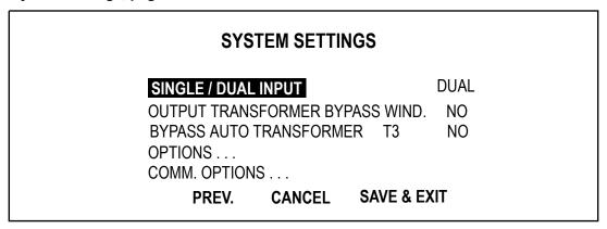
The Single / Dual Input Screen is password protected. (See **3.2 - Security Access and Passwords** for more information on Security Access and Passwords.) After highlighting Single / Dual Input from the System Settings Screen, and pressing SELECT, the following screen will appear.
